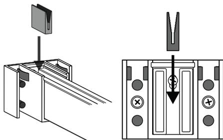
**STEP 1:** Insert Base between the rails of the Header Bar.
