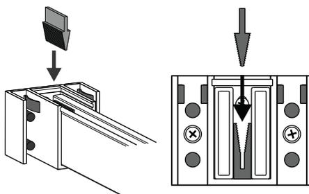
**STEP 2:** Push the Wedge into the Base until it forces to the rails of the Header Bar against the sides of the header block.
