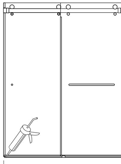
Apply a Single Bead along inside and outside of Soft Sill and Center Guide
