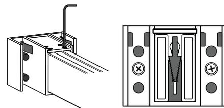
**STEP 3:** Insert the Header Bracing plate into the slot of the Header Block and tighten the set screws
