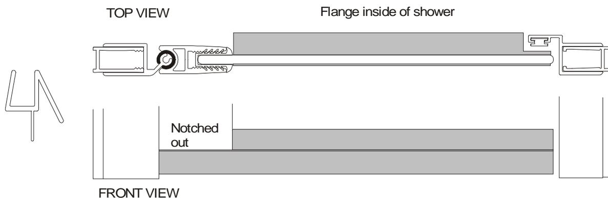
11. Run a continuous bead of silicone across the outside of the shower unit where the metal meets the walls and threshold.
