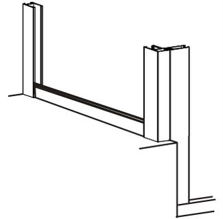
4. Insert setting blocks, then insert panel into the panel sill and into back wall channel. Adjust as necessary. Insert corner post over edge of glass and end of panel sill. Realign the corner post to the hole drilled earlier. Secure post with #8 X 1-1/2 FHPHMS. Temporarily hold post to glass with painters tape.
