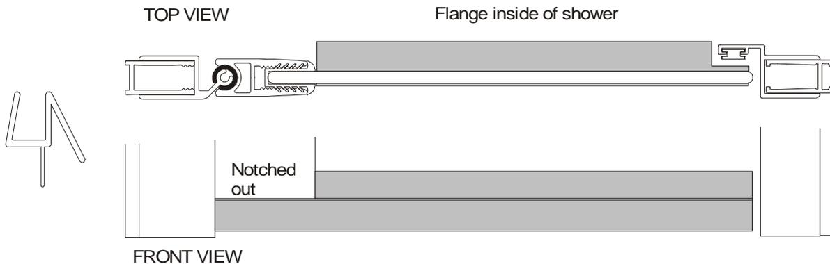
10. Run a continuous bead of silicone around the outside of the unit where the metal meets the walls and threshold
