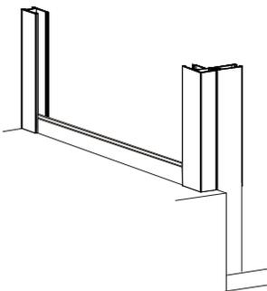
4. Using setting blocks, insert panel into the panel sill and into back wall channel. Adjust as necessary. Insert corner post over edge of glass and end of panel sill. Realign the corner post to the hole drilled earlier. Secure post with #8 X 1-1/2 FHPHSMS. Plumb the 90° post and temporarily hold post to glass with painters tape.
